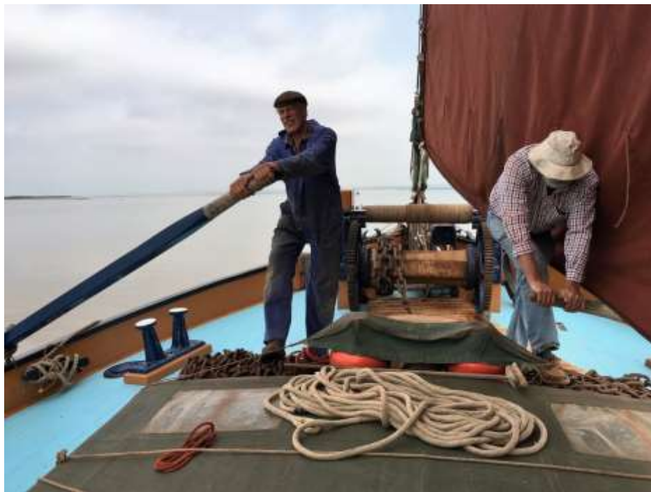
Using the sweeps when the wind is no longer moving the boat
